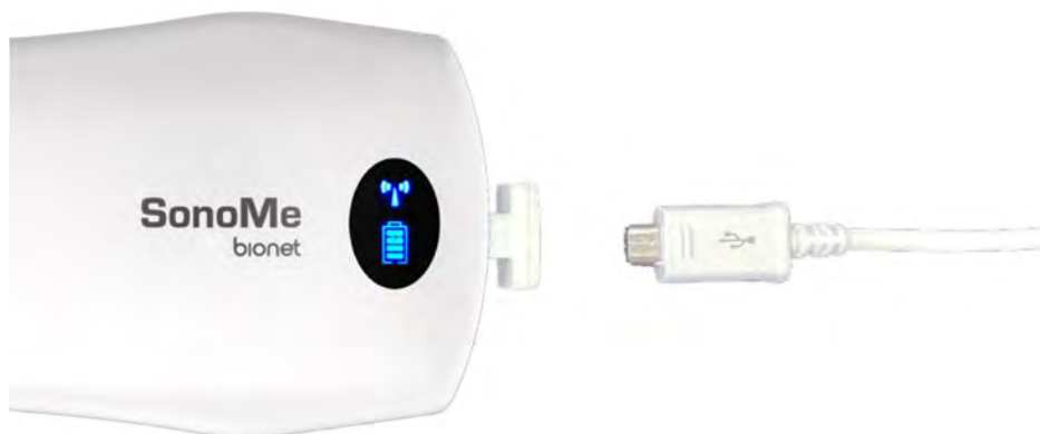
[Figure 5-1] Probe Charging via USB Cable
